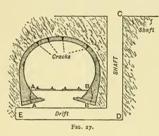
covered from A to A and from B to B. This reduced the bearing area of the tunnel walls at A and B to one half, with the result that the arch of the tunnel was being forced by the superin-
